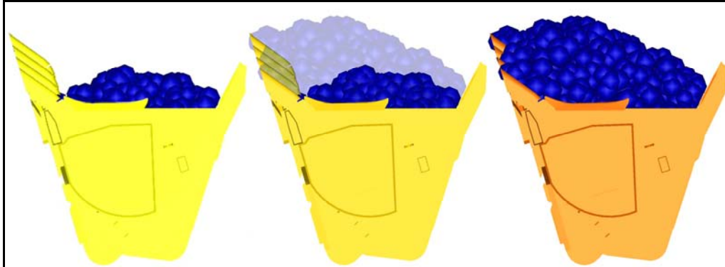
Figure 7 Comparison of Heaped 2:1 vs. scooped pile
